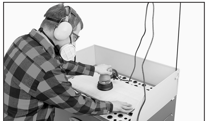
Figure 14. Typical sanding operation set up.
